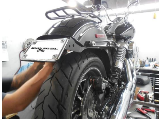
Mounting Bracket Installed
