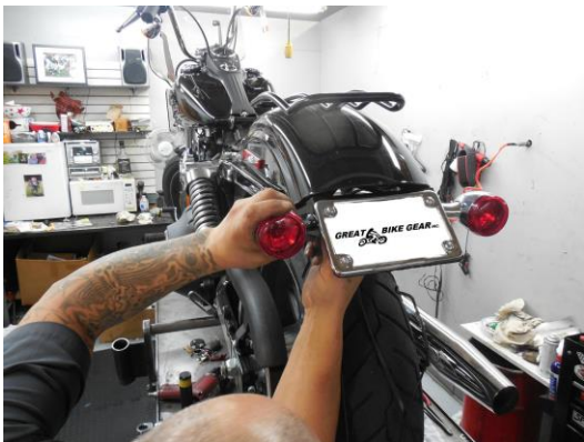
Turn Signals Installed
