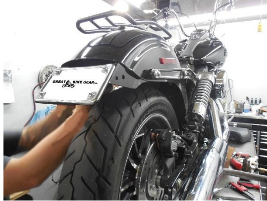
Mounting Bracket Installed
